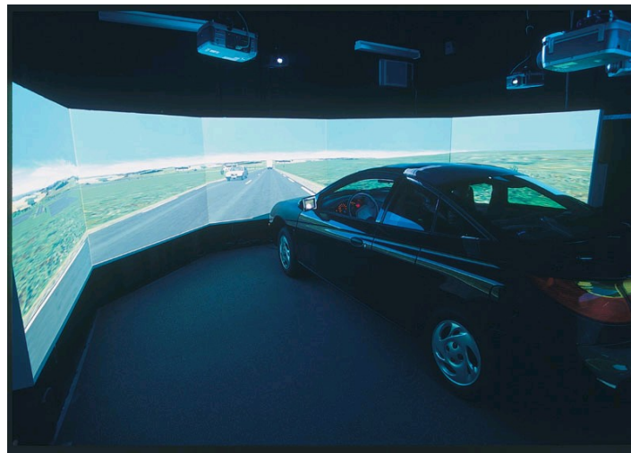
Figure 3.1 HumanFIRST full-cab driving simulator set up
