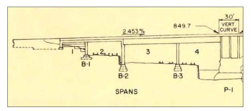
Figure 43. West Approach Span Layout
