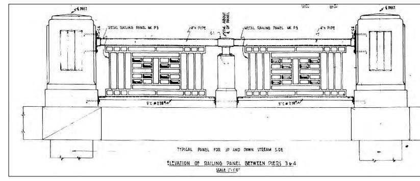
Figure 51. 1939 to Present Aluminum Railing with Concrete Pilasters
