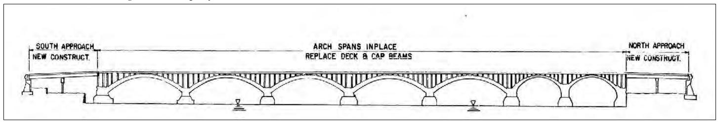
Figure 55. Completed 1979 Rehabilitation
