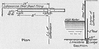
FIG. 5. SUPPORT FOR BOTTOM OF STEEL SHEETING FOR COFFER-DAM
