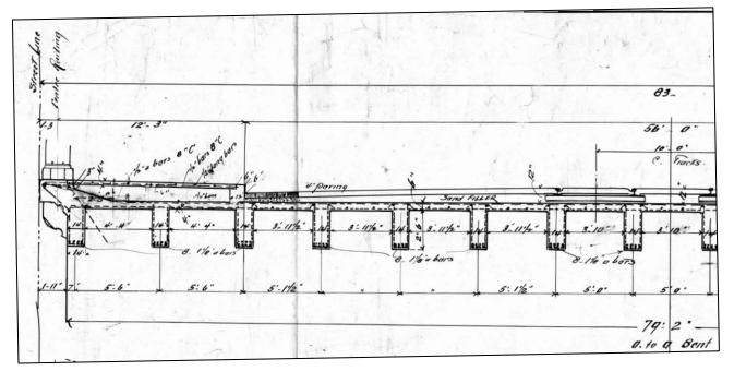
Figure 46. Half Section of 1917 Concrete Approach Spans
