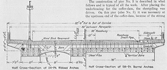
FIG. 3. CROSS-SECTION OF THE CONCRETE ARCH BRIDGE AT THIRD AVE., MINNEAPOLIS, MINN.
