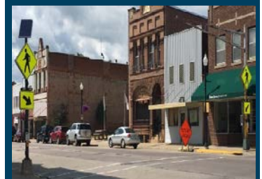
Push button and motion activated, LED-enhanced crossing system in Sleepy Eye, MN (1 st Ave / HWY 14)
