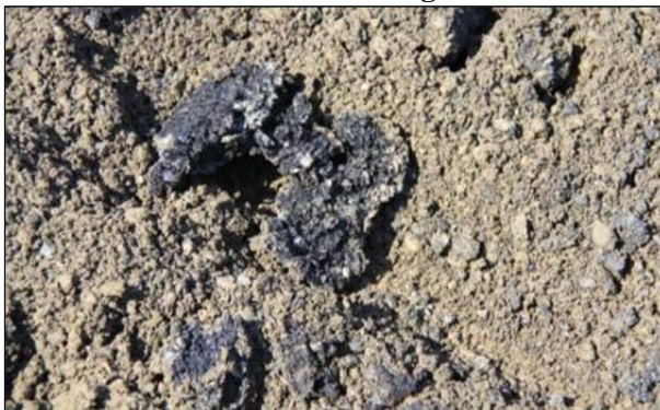
Figure 3.6: FDR-NS: Chunks at start of test pulverization.
