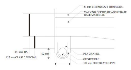
Figure 1. Edge drain configuration to simulate retrofitting a JCP overlying a dense graded base with edge drains (Roberson & Birgisson 2000)
