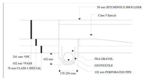
Figure 2. Typical edge drain configuration with edge drains (Roberson & Birgisson 2000)
