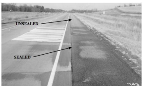
Figure 3. Two concrete test sections after rain (Olson & Roberson 2003).
