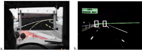
Figure 1. a. Typical view of roadway and b. HUD view of roadway (from MnDOT 2004-09)
